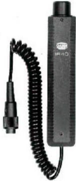
Contactless temperature measurement from -20 to +199.9 °C, resolution 0.1 °C, emissivity permanently set at 95 %, ratio of measured area to distance 2.5:1 (Ø 45 mm at a distance of 100 mm), sensor length 185 mm x 36 x 33 mm, coiled cable 320/1200 mm.
